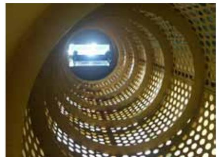
*The perforated screening metal sheets are bolted to the rotary frame and easily replaceable*
