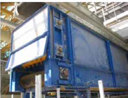
Dosing reels by the discharge side
