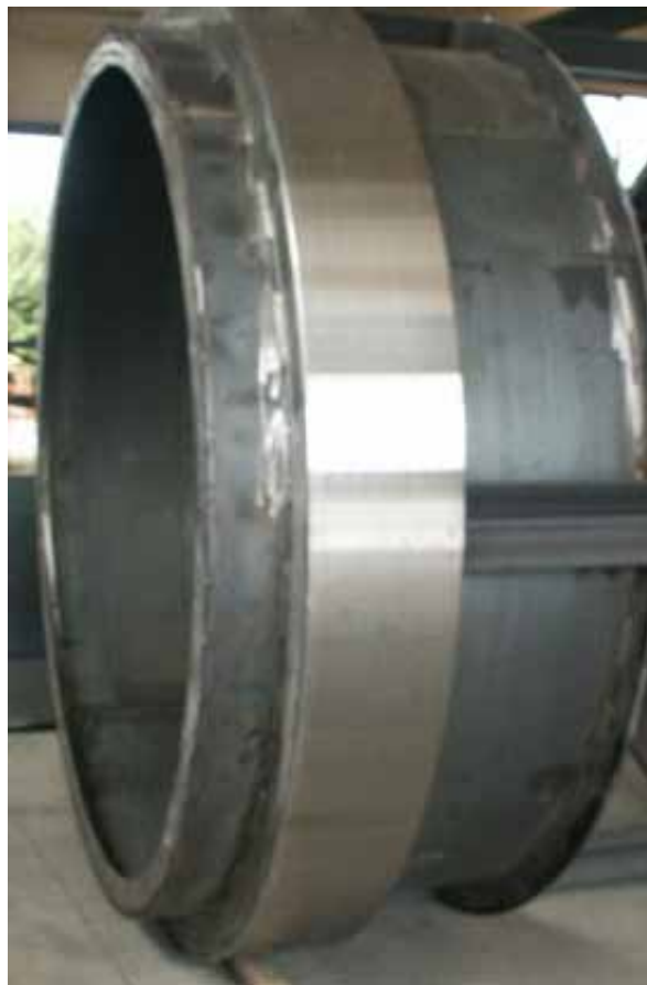
Silent rotation, without vibrations and less wear of sliding wheels are given by machine-lathed roller paths.
