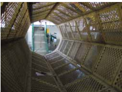
The perforated screening metal sheets are bolted to the rotary frame and easily replaceable
